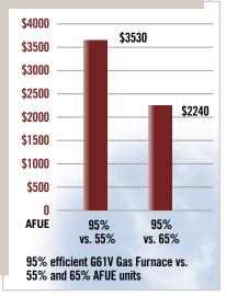
This chart depicts potential energy savings you can expect from the G61V furnace, versus older furnaces with lower efficiency ratings. Criteria used in this example are 2,000 full-load heating hours, with a 60,000 Btuh heating design load and \$1.281 ccf for gas. Your actual savings may vary, depending on the weather patterns in your local area, local fuel rates and your individual lifestyle.
