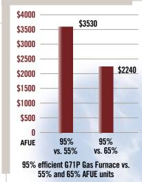
This chart depicts potential energy savings you can expect from the G71P furnace, versus older furnaces with lower efficiency ratings. Criteria used in this example are 2,000 full-load heating hours, with a 60,000 Btuh heating design load and \$1.281 ccf for gas. Your actual savings may vary, depending on the weather patterns in your local area, local fuel rates and your individual lifestyle.
