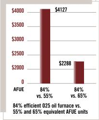
This chart depicts potential energy savings you can expect from the 025 furnace versus older furnaces with lower efficiency ratings. Criteria used in this example are 2,000 full-load heating hours, with a 80,000-Btuh heating design load and \$1.90 per gallon for oil. Your actual savings will vary depending on the weather, local fuel rates and your lifestyle.
