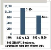
This chart compares the 5-year savings you can expect from an HP13 heat pump vs. units with lower efficiency ratings, based on a 36,000 Btuh/3-ton unit (EPA Region 9). Your actual savings will vary depending on the weather, local fuel rates, indoor coil and your lifestyle.
