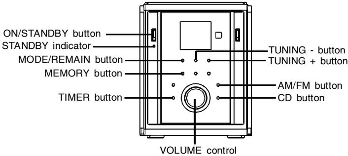
You can set the timer to wake you up at a certain time. Before setting, please select your choice of source (AM, FM station, or CD disc). Press the ON/STANDBY button to make sure the STANDBY indicator is steadily on and the current time will show in the display.
