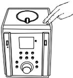
Open the CD door by pressing PUSH OPEN area and push a CD disc down onto the center spindle. The label side of the CD should face upward.
