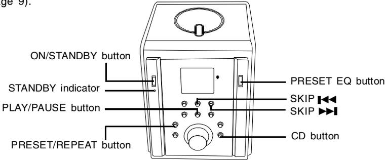
1. Press the ON/STANDBY button, the STANDBY indicator will go off and the display will light up.
