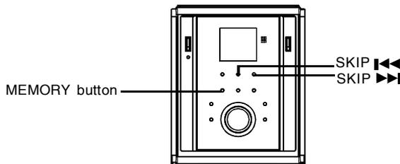
1. During **stop** mode, press the MEMORY button, the words **MEMORY** and **TRACK** will be steadily on in the display. The symbol "Pr:01 --" also will show in the display.
