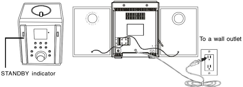
**NOTE:** If the plug of the AC power cord does not match your outlet, do not force it. Reverse it and try again. This plug is polarized and only fits one way into the wall outlet.
