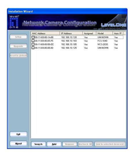
For more detailed usage of the Installation Wizard, please refer to the user manual of the Installation Wizard included in the product CDROM to find the location of the Network Camera. There may be many Network Cameras in the local network. Users can differentiate the Network Cameras with the MAC address. The MAC address is printed on the back of the Network Camera body. Initial Access to the Network Camera
