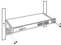
Figure 2. Mount the Switch in the rack
