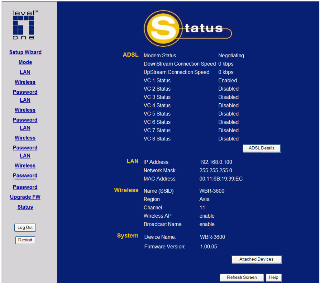
Figure 67: Status Screen - Bridge Mode
