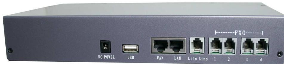
1. DC Power            12Volt DC / 1A Power Adaptor with 100~240V AC power input
