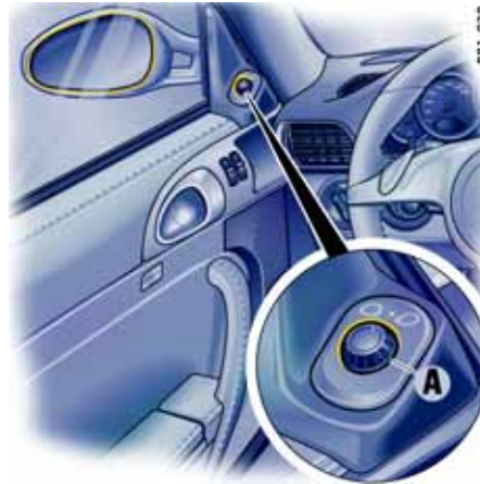
A - Control switch for door mirror adjustment
