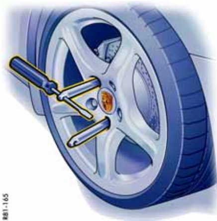
Screw in two assembly aids for vehicles with Porsche Ceramic Composite Brake
