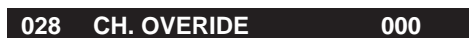
After Master TV setup has been completed, set Installer menu item 028 Ch Override to 000.
