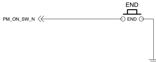
Figure 1.20 END Keypad Circuit
