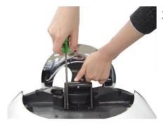
**2.** Separate the stand base using a screwdriver as shown in the picture.
