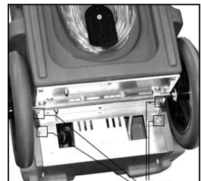
Pump removal, location of 4 bolts
