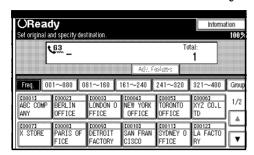
E Press the destination key If the desired destination key is not shown, press [▲] and [▼] to look through the table.
