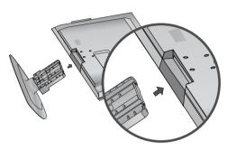
Fix the 4 bolts securely using the holes in the back of the TV.
