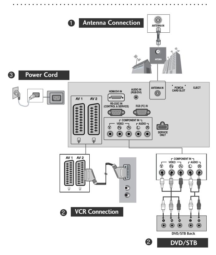
\* To connect an additional equipment, see the External equipment Setup section in CD Manual.
