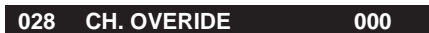
After TV setup has been verified, set item 028 Ch Override back to 000.
