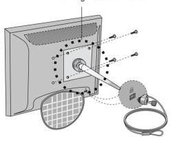
Kensington Security Slot- optional Connected to a locking cable that can be purchased separately at most computer stores
