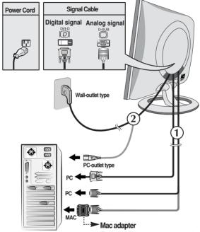
For Apple Macintosh use, a separate plug adapter is needed to change the 15 pin high density (3 row) D-sub VGA connector on the supplied cable to a 15 pin 2 row connector.
