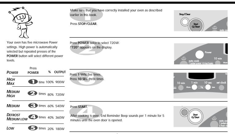
Your microwave oven is equipped with 5 power levels to give you maximum flexibility and control over cooking. The table below shows the examples of food and their recommended cooking power levels for use with this microwave oven.
