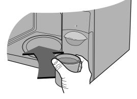
Press the START button six times to set 3 minutes of cooking time. You will hear a BEEP each time you press the button. Your oven will start before you have finished the sixth press; don't worry this is normal. The **DISPLAY** will count down from 3 minutes. When it reaches 0, BEEP sounds. Open the oven door and test the temperature of the water. If your oven is operating the water should be warm. **Be careful** when removing the container it may be hot.
