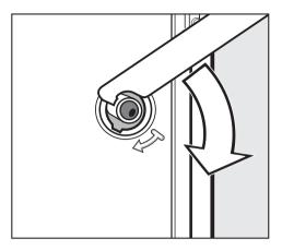
Turn the right shipping strut clockwise 90° with the enclosed combination wrench.
