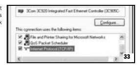
Click Properties button, then choose IP Address tab. Select Obtain an IP address automatically. Press OK. You have completed the client settings. (Figure 34)
