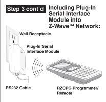
NOTE: Programmer/Remote must be in close proximity to Plug-In Serial Interface Module when including into network
