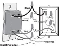
This wire is used in 3-way installations only. For single pole installations, do not remove this insulating label.
