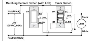
**NOTE:** The timer switch **must** be installed in a wall box that has a Load connection. The matching remote switch **must** be installed in a wall box with a Line Hot connection and a Neutral connection. A Neutral wire to the matching remote switch needs to be added as shown.
