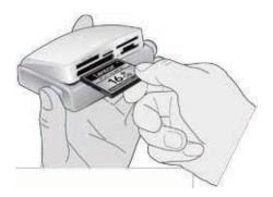
**WARNING:** Do not remove the card from the reader when the LED activity light is blinking or you may lose data or damage the card.
