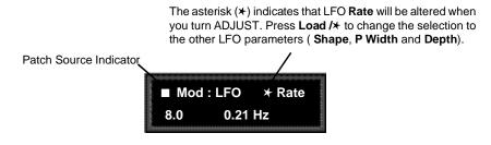
The display now shows position 8.0 in the Edit matrix Mod Row. The small square in the upper left corner of the display is a *patch source indicator*. This indicator appears whenever a modulator (such as the LFO in this example) has been assigned as a patch Source in the effect being edited.
