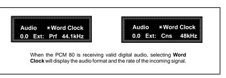
When External clock is first selected, the PCM 80 will repeatedly try to establish lock. You can choose to have any subsequent interruptions of the incoming digital audio signal dealt with in one of two ways. An Auto Lock feature allows you to choose to have the PCM 80 attempt to re-establish lock, or not. (See 0.3 Auto Lock.) In either case, the PCM 80 will immediately mute the digital input, and switch to Internal clock at the sample rate of the last valid external signal.
