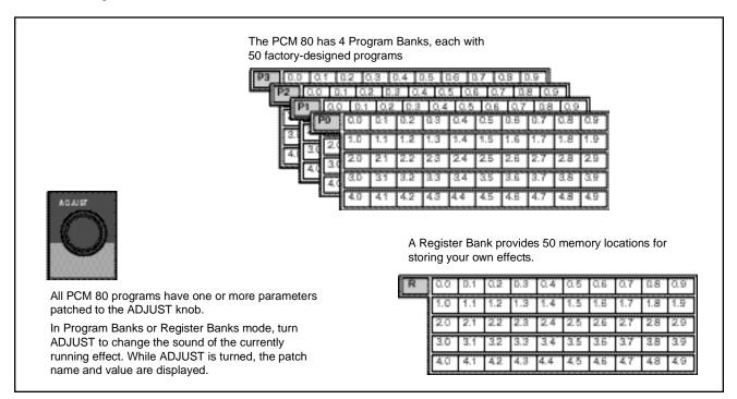
The procedure for loading effects is the same, whether you are choosing from banks of factory presets, or from your own banks of registers. When first turned on, the PCM 80 will load whatever effect was running when it was last turned off. When shipped from the factory, the first effect in the first Program Bank (**P0 0.0 Prime Blue**) is loaded. The Bank ID (**P0, P1, P2, P3**),matrix location, program name, and the algorithm from which the effect is derived are all displayed.
