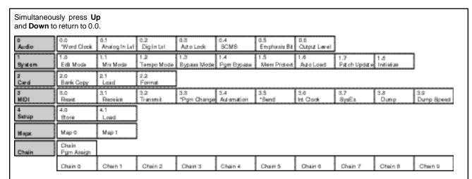
An asterisk (\*) accompanying a parameter name indicates that there are subparameters available at that matrix location. The **Load** /\* LED will light whenever an asterisk appears in the display. Press **Load** /\* to step to the next subparameter. From any point in the matrix, press **Up** or **Down** together with **Load** /\* to backstep to the previous parameter.
