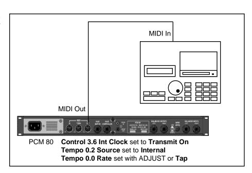
The configuration below shows the MIDI connections for controlling the PCM 80 simultaneously with MIDI Clocks from a sequencer, and messages from another MIDI controller. Note that the controller is set to "local control off" and the sequencer is set to "echo input".
