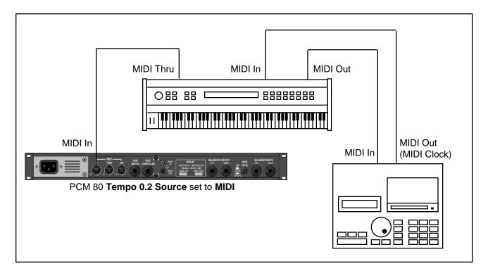
Two PCM 80s can be slaved together by connecting a cable from the MIDI OUT jack of the master to the MIDI IN jack of the slave. Additional PCM 80s can be slaved to the master by connecting a cable from the MIDI THRU port of one slave unit to the MIDI IN port of the next unit. All of the PCM 80s must be set to the same MIDI channel.
