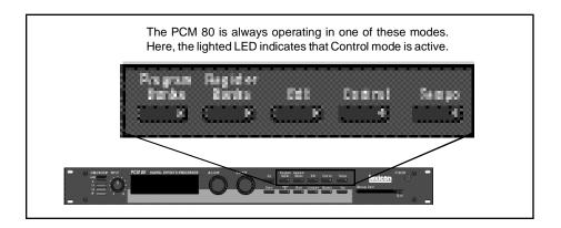
The five mode buttons give you the first level of access to all of the functions and parameters in the PCM 80.
