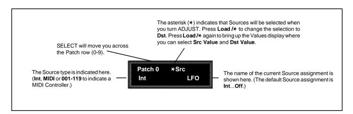
Pressing the Load /★ button will change the display to allow you to sequentially select: Src, Dst, Src Value and Dst Value. Press Up or Down together with Load /★ to backstep to the previous parameter.
