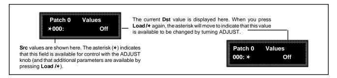
This display allows you to assign Destination values to specific Source values. These assignments are made in pairs, each with a value for the Source and a value for the Destination. For example, the default is two pairs mapped as follows:
