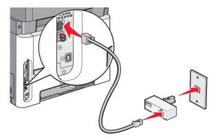
**3** Connect the answering machine or telephone to the adapter. Use one of the following methods:
