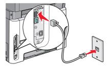
**3** Remove the protective plug from the printer EXT port **3**.
