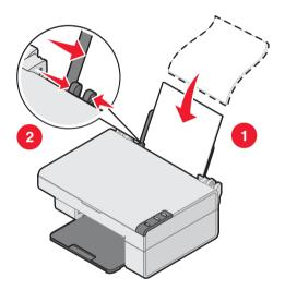
2 Squeeze the release tab, and slide the paper guide to the right until it rests against the edge of the paper.
