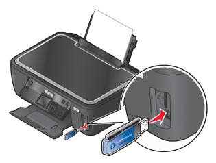
Bluetooth Dongle Connected appears on the display.
