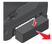
**CAUTION—POTENTIAL INJURY:** The area behind the duplex cover has protruding ribs as part of the paper path. To avoid injury, use caution when accessing this area for clearing a paper jam.
