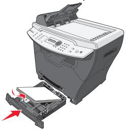
6 Make sure the paper is below the maximum fill lines on the left inside wall of the tray.
