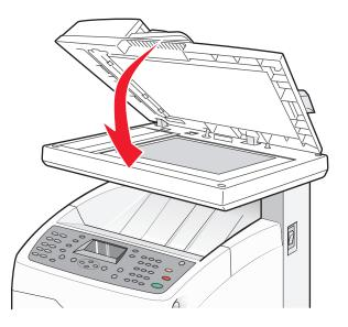
7 When all the jammed paper is removed, **Return the Removed Original and Press Start** appears. Place the original document in the ADF, and then press **Start**  $\diamondsuit$  to continue with the scan job.
