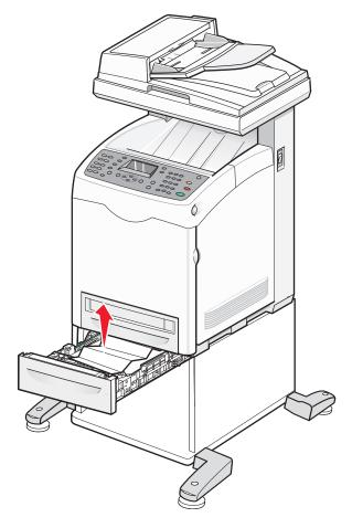
• Jams behind the tray area—Locate the jam on the bottom surface of the tray housing. You may have to reach far under the printer to locate the jam, as shown in the following illustration. Pull the jam straight out.
