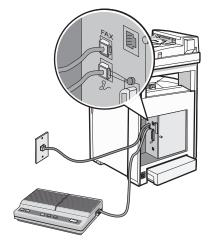
**Note:** Once this plug is removed, any country- or region-specific equipment that you connect to the printer by the adapter, as shown, will not function properly.
