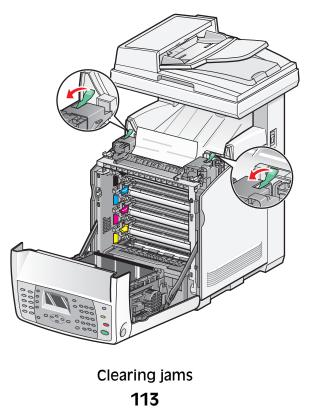
**3** Lift the fuser cover, and then remove the jammed paper.
