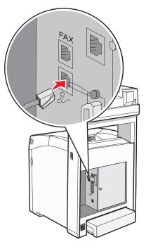
**3** Connect the other end of the telephone cord into an active telephone wall jack.
