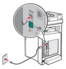
**3** Remove the protective plug from the EXT port  $\mathcal{L}$  of the printer.
