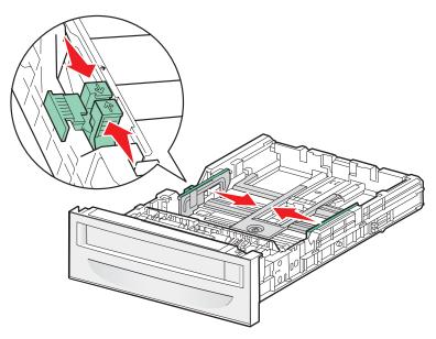
Note: Notice the load line label on the side of the tray which indicates the maximum stack height for your paper.
