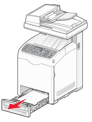
**6** Remove any jammed paper from inside the tray housing.
