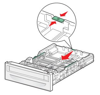
**3** Squeeze the width guide tabs together as shown, and slide the width guide to the correct position for the paper size being loaded.
