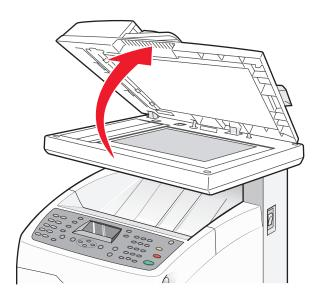
**3** Move the scanner lock switch to the unlocked position.
