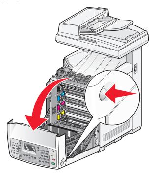
**2** Pull out the jammed paper from the duplex unit. If jammed paper cannot be found, go to the next step.
