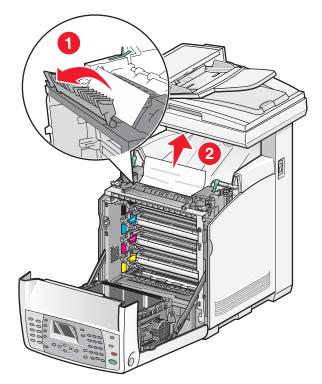
4 Close the fuser cover, and then lower the pressure release levers.
