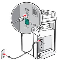
**3** Remove the protective plug from the EXT port  $\mathcal{J}_{\sim}$  of the printer.
