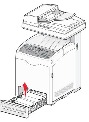
• Jams behind the tray area—Locate the jam on the bottom surface of the tray housing. You may have to reach far under the printer to locate the jam, as shown in the following illustration. Pull the jam straight out.
