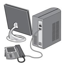
**5** Connect a third telephone cord from the computer modem to the EXT port  $\mathcal{J}_{\sim}$  of the printer.
