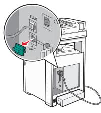
**4** Connect a second telephone cord from the telephone to the computer modem.
