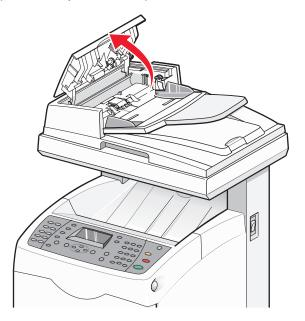
2 If the jam is in the paper feed area, remove the jam by carefully pulling it up.
