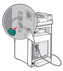
**4** Connect the other telephone cord to a telephone, and then plug it into the EXT port  $\mathcal{J}_{\mathcal{T}}$  of the printer.
