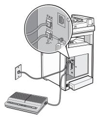
**Warning—Potential Damage:** Do not touch cables or the printer in the area shown while actively sending or receiving a fax.
