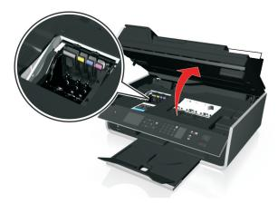
**Note:** The printhead moves to the cartridge installation position.
