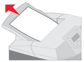
Clearing jams between the fuser and the standard bin 73
