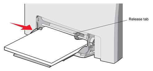
Make sure the media fits loosely in the multipurpose feeder and is not bent or wrinkled.
