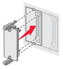
**Note:** The entire length of the connector on the card must touch and be flush against the system board. Be careful not to damage the connectors.
