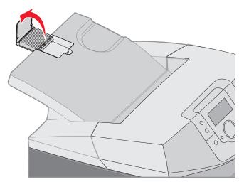
To close the media stop, fold the extension forward and down. Raise the media stop, and then fold it back down into its closed position.
