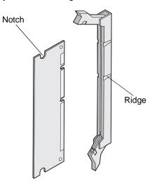
**5** Push the memory card straight into the connector until it *snaps* into place. Make sure each latch fits over the notch located on either side of the memory card.
