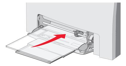
Identifying the multipurpose feeder or the manual feed slot **55**
