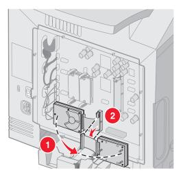
3 Replace the metal plate. See Replacing the system board metal plate.
