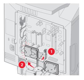
9 Replace the metal plate. See **Replacing the system board metal plate**.
