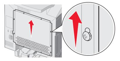
**3** Pull the metal plate forward to remove it.
