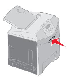
2 Open the upper door fully. Grasp the handle on the inner door and pull to open both the inner and lower doors. Gently lower the lower door. Now the photoconductor units can be seen.
