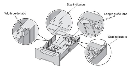
**Note:** If the same media size is loaded again, the tray does not need to be completely removed from the support unit. Just remove it partially and load the media without adjusting the guides.
