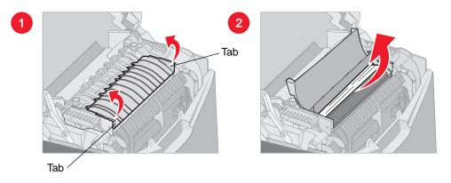
If the jammed media is partially under the fuser and partially exposed from the slot behind the fuser, the operator panel indicates a 202.xx Paper Jam.
