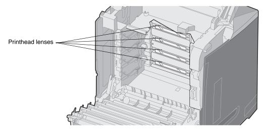
5 Clean the lenses using a can of compressed air (same as the compressed air used to clean a camera lens).
