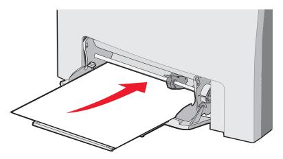
12 Slide the width guide to the right until it lightly touches the edge of the stack for transparencies, card stock, or envelopes. For paper, the guide was already placed before the paper was loaded; however, check to see if the guide needs a slight adjustment.
