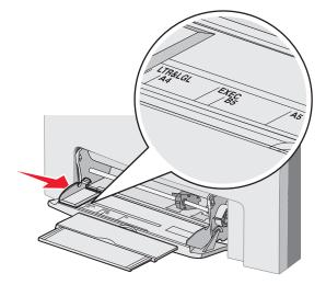
Identifying the multipurpose feeder or the manual feed slot 52
