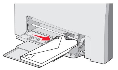
Warning: Never use envelopes with stamps, clasps, snaps, windows, coated linings, or self-stick adhesives. These envelopes may severely damage the printer. Do not feed stamped envelopes into the multipurpose feeder. The stamp is shown in the illustration only for placement.
