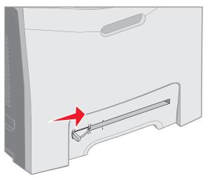
2 Load one sheet of media. Load the media so it fits flush with the right side of the manual feed slot.
