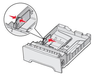
3 Squeeze the length guide tabs together as shown, and slide the length guide to the correct position for the size of paper being loaded. For setup, load Letter or A4 based on the standard size for your country or region. Notice the size indicators on the bottom of the tray on both sides of the guide. Use these indicators to help position the guide at the correct size. Notice the load lines on the width guide tab which is the maximum height indicator for loading media.
