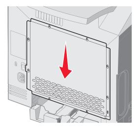
Replacing the system board metal plate **122**
