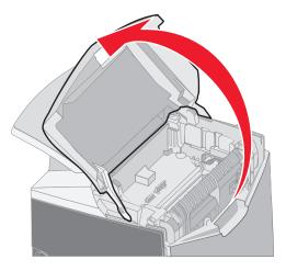
Replacing the fuser after long-term storage 87
