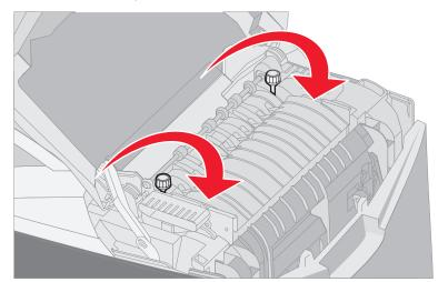
Warning: Make sure the thumbscrews are tightened fully before closing the upper door.
