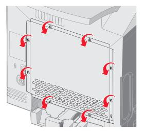
2 Lift the metal plate up until each screw is in the keyhole.
