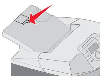
2 Lift it up and back until it is flat at a 180 degree angle.
