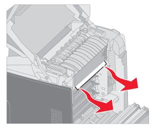
Clearing jams under the fuser or fuser cover 71
