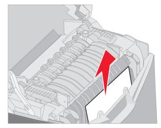
**Note:** If most of the jammed media is not visible with the upper door open, open the lower door to access the jam. To open the lower door without also opening the inner door, pull on the lower door handle. Do *not* pull the inner door handle, or both the inner door and the lower door will pull down together.
