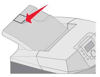
2 Lift it up and then back until it stops at a 90 degree angle.
