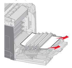
3 If the media does not pull free at all, remove all four photoconductor units. (If help to remove them is needed, see the illustration on **page 31**.) Remove the jammed media, then reinstall the photoconductor units.
