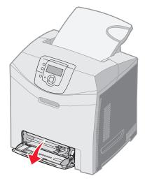
Identifying the multipurpose feeder or the manual feed slot **51**
