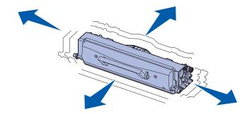
5 Install the new toner cartridge by aligning the white rollers on the toner cartridge with the white arrows on the tracks of the photoconductor kit and pushing the toner cartridge in as far as it will go. The cartridge *clicks* into place when correctly installed.
