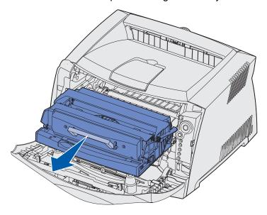
**Warning:** Do not leave the print cartridge assembly exposed to direct light for an extended period of time. Extended light exposure can cause print quality problems.
