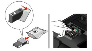
**Note:** Install the new ink cartridges immediately after removing the protective cap to avoid exposing the ink to air.
