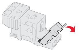
**9** Push the cartridge holder firmly into the stapler until the cartridge holder *clicks* into place.
