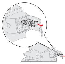
**5** Use the metal tab to lift the staple guard, and then pull out the sheet of staples.
