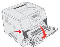
**2** Push the release latch, and open the top front cover.
