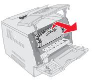
Warning: Do not touch the photoconductor drum on the underside of the cartridge. Use the cartridge handle whenever you are holding the cartridge.
