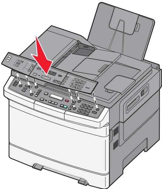
If needed, change the language on the printer control panel cover by removing the cover, and then install the cover for your language.
