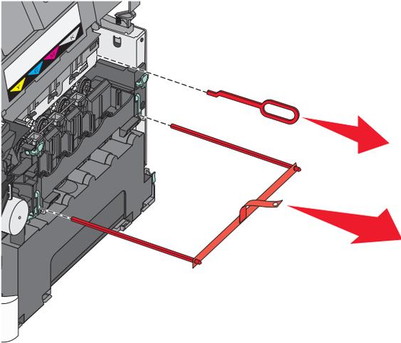
Remove the packing rods and clip.
