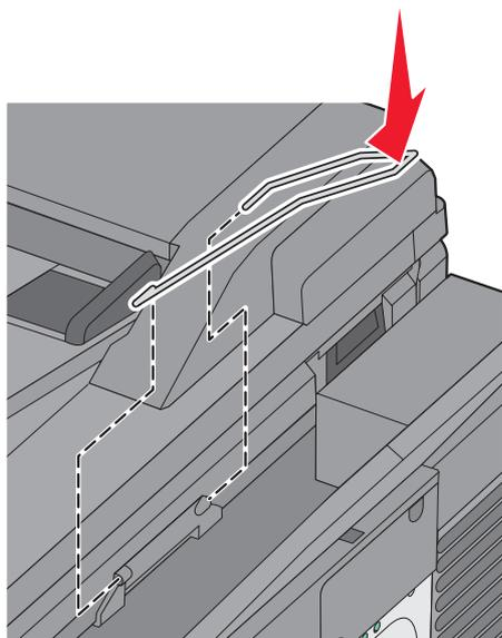
Attach the ADF tray, the exit tray, and the paper bail to the printer.
