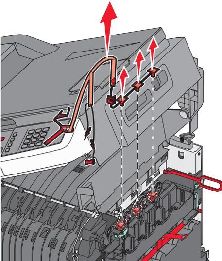
Remove the red and orange packing material.
