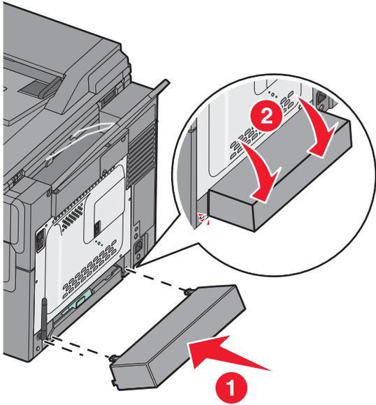
Attach the paper tray cover to the rear of the printer.
