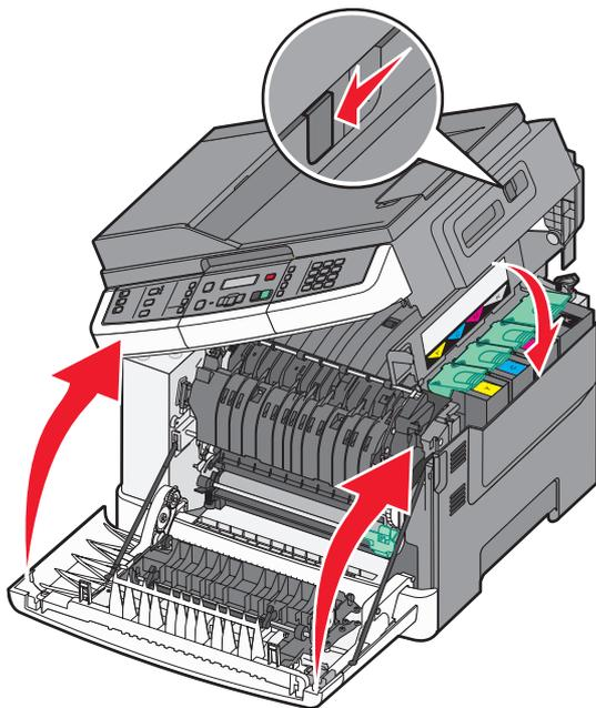
Install the side panel, slide the latch to the left and close the top cover. Close the front door.
