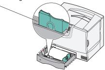
**6** Squeeze the front guide lever and slide the guide until it firmly touches the stack of paper.
