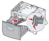
**3** Squeeze the two front guide levers and slide the guide to the correct position for the size paper you are loading.
