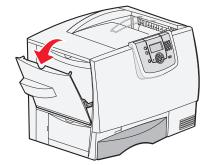
**2** Squeeze the paper guide lever and slide the guide all the way toward the front of the printer.
