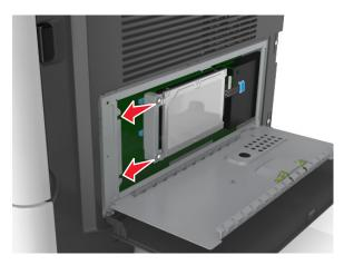
**d** Tighten the two screws.
