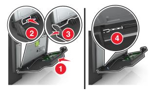
**10** Run the ISP cable through the controller board shield.
