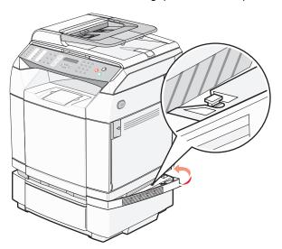
**3** Align the other bracket with the hole on the left side of the printer as shown. Press the bracket flat against the printer, and then tighten the thumbscrew.
