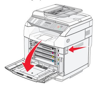
**3** Remove the toner cartridges one at a time.
