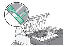
Warning: Do not pull the jammed paper out from the bottom of the ADF.
