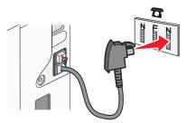
**4** If you would like to use the same line for both fax and telephone communication, connect a second telephone line (not provided) between the telephone and the F slot of an active telephone wall jack.
