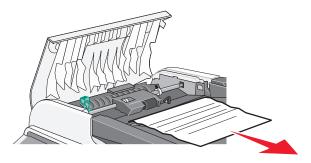
4 Lower the tension release lever back into place until it locks.
