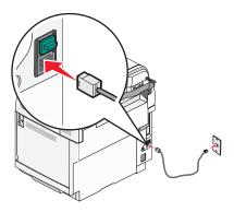
**3** Remove the protective plug from the EXT port  $\widehat{\ }$  of the printer.
