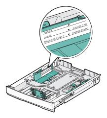
**3** Squeeze the width guide tabs together as shown, and slide the width guide to the correct position for the paper size being loaded.
