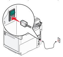
**3** Remove the protective plug from the EXT port  $\stackrel{\frown}{=}$  of the printer.
