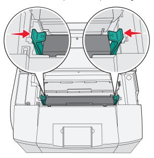
**6** Grasp the handle, and pull the photodeveloper cartridge straight up and out.
