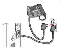
**5** If you would like to use the same line for recording messages on your answering machine, connect a second telephone line (not provided) between the answering machine and the other N slot of the telephone wall jack.
