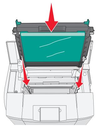
11 Push the latches away from each other to lock the photodeveloper cartridge into place.
