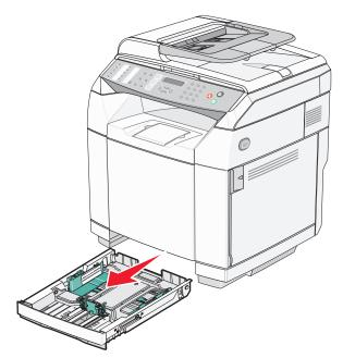
2 Using a coin or a flat head screwdriver, unlock the tray on each side.
