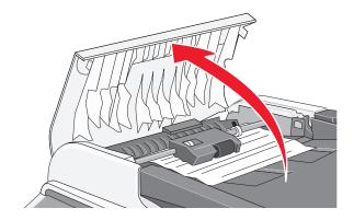
**2** Lift the tension release lever so that it is in the up position.
