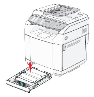
• Jams behind the tray area—Locate the jam on the bottom surface of the tray housing. You may have to reach far under the printer to locate the jam, as shown in the following illustration. Pull the jam straight out.
