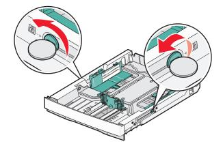
**3** Fully extend the tray until the locking tabs are in the LGL position.
