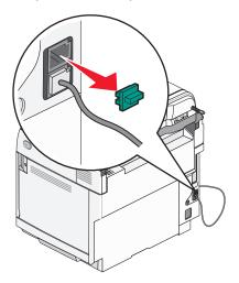
**4** Connect the other telephone cord to a telephone, and then plug it into the EXT port  $\widehat{\ }$  of the printer.
