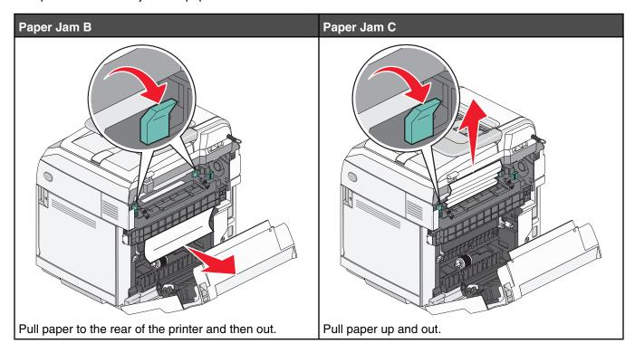
**Note:** Gently pull the paper out to avoid tearing it. Whenever possible, pull the paper towards the bottom of the printer to avoid contaminating the fuser.
