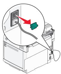
**4** Connect a second telephone cord from the telephone to the computer modem.
