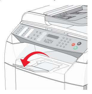
The paper support is inclined so the paper now remains in a neater stack in the standard exit bin.
