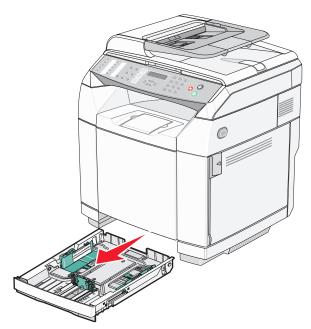
2 Squeeze the length guide tabs together as shown. Slide the guide to the correct position for the paper size being loaded.
