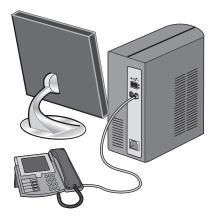
**5** Connect a third telephone cord from the computer modem to the EXT port of the printer.
