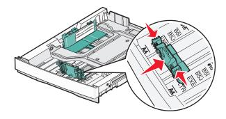
**Note:** Notice the size indicators on the bottom of the tray on both sizes of the guide. Use these indicators for help positioning the guide.
