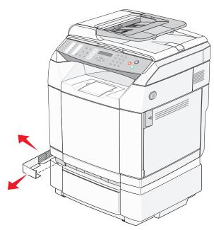
**5** Loosen the right thumbscrew, and remove the right bracket.
