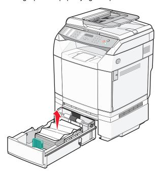
• Jams behind the tray area—Locate the jam on the bottom surface of the tray housing. You may have to reach far under the printer to locate the jam, as shown in the following illustration. Pull the jam straight out.
