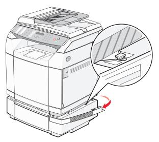
4 Remove the left side cover by starting at the back of the printer and gently pulling each of the four slots off of its matching tab as you work your way to the front of the printer.
