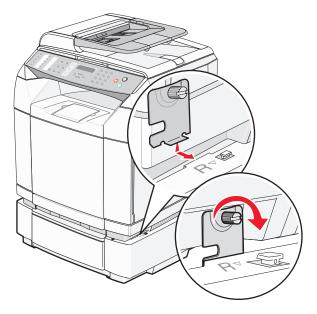
2 Starting at the front of the printer, push the right side cover onto the printer, fitting each slot on the cover over its corresponding tab on the drawer in order to cover the gap between the printer and the drawer.
