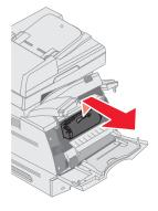
Warning: Do not touch the photoconductor drum on the underside of the cartridge.
