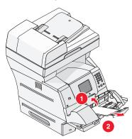
If the jammed envelope has entered the MFP and cannot be pulled out, remove the envelope feeder.
