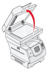
**4** Open the scan unit access door, and remove any jammed pages.
