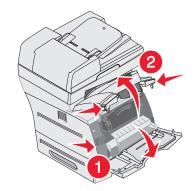
3 Lift and pull the print cartridge out of the MFP.
