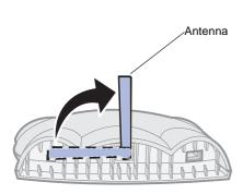
**Note:** Rotate the antenna clockwise from the back.
