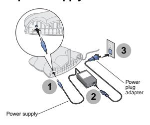
If necessary, replace the power plug adapter with the correct power plug adapter for your geography.
