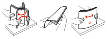
5 Load the paper stack with the recommended print side faceup. Load the stack toward the back of the tray as shown. When loading preprinted letterhead, place the header toward the front of the tray.
