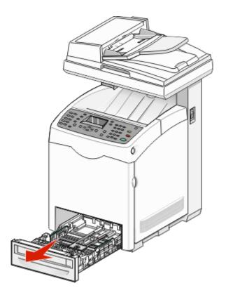
**2** Squeeze the length guide tab as shown. Slide the guide to the correct position for the paper size being loaded.
