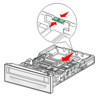
**3** Squeeze the width guide tabs together as shown, and slide the width guide to the correct position for the paper size being loaded.
