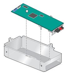
**8** Attach the ISP to the metal housing using two thumbscrews.
