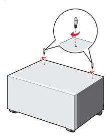
**4** Align the optional tray to the printer stand, then lower the printer to the tray.
