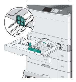
**2** Make sure to release the width guide lock at the rear of the tray. Squeeze and then slide the width guide to the correct position for the paper size you are loading.
