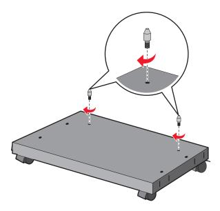
**5** Align the trays to the caster base, then lower the printer to the trays.
