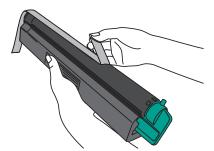
Insert the new cartridge into the printer and then turn the toner lock lever to the left.
