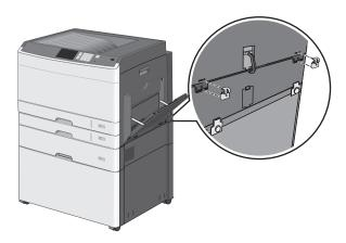
**d** Secure the brackets with screws.
