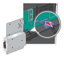
**13** Reconnect the fan cable to its connector on the system board.
