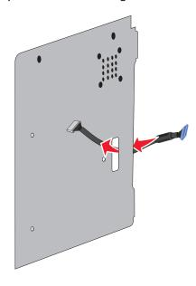
**10** Attach the ISP cable to the connector on the ISP.
