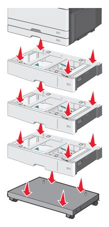
**6** Lock the standard and optional trays together using the brackets that came with the optional tray.
