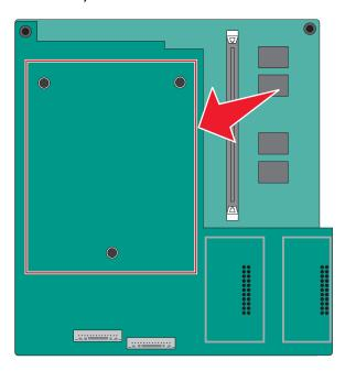
**4** Align the standoffs of the printer hard disk to the holes on the system board, and then press on the printer hard disk until the standoffs are in place.
