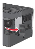
2 Turn the screws on the metal panel counterclockwise to remove them, and then pull the panel down.
