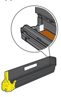
**5** Reinstall the imaging unit. When inserted into the printer, the LED wipe will rub across the row of LEDs, thus cleaning the printhead lenses.
