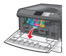
**b** Push the imaging unit lock lever up and pull out the imaging unit.
