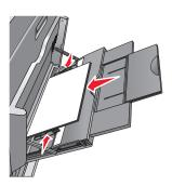
**Warning—Potential Damage:** Never use envelopes with stamps, clasps, snaps, windows, coated linings, or self-stick adhesives. These envelopes may severely damage the printer.
