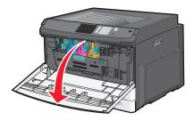
**Warning—Potential Damage:** To avoid overexposing the imaging units, do not leave the door open for more than 10 minutes.
