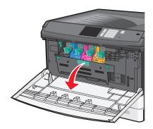
3 Push the imaging unit lock lever up and pull out the imaging unit with the toner cartridge attached to it.
