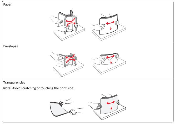
4 Load the paper or specialty media. Slide the stack gently into the multipurpose feeder until it comes to a stop.
