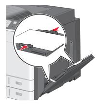
**6** From the printer control panel, set the Paper Size and Paper Type for the multipurpose feeder (MP Feeder Size and MP Feeder Type) based on the paper or specialty media loaded.
