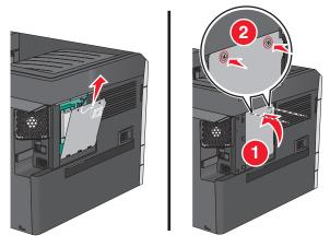
**b** Turn the screws on the metal panel clockwise.
