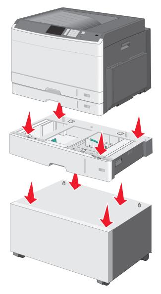
**5** Lock the standard and optional trays together using the brackets that came with the optional tray.
