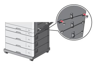
**d** Secure the brackets with screws.
