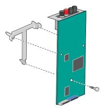
**7** Insert the ISP into the metal housing.
