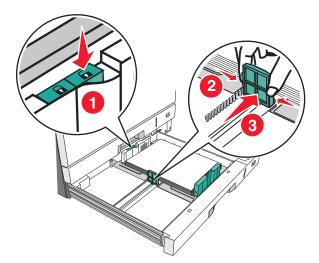
**Note:** Always use the width guide lock at the rear of the tray to prevent the margins from being knocked out of adjustment.
