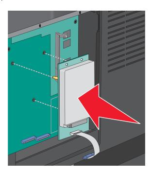
**5** Insert the plug of the printer hard disk interface cable into the receptacle of the system board.
