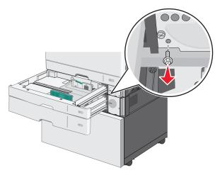
**c** Place a bracket over the screw hole and secure it with the screw.
