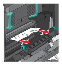
**b** If the paper is not visible, then you will need to remove the fuser unit.
