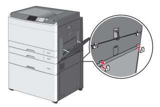
**b** Secure the brackets with screws.
