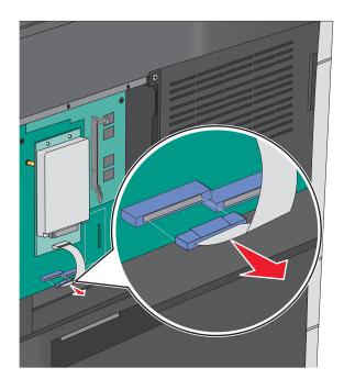
**3** Remove the printer hard disk.
