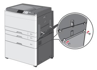
**c** Insert brackets on the slots located at the back of the printer and optional tray.
