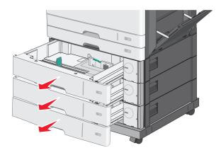
**b** Reach into the lower optional tray and insert a screw, pushing it upward to the optional tray above it.
