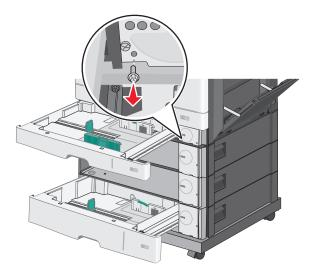
**c** Place a bracket over the screw hole and secure it with the screw.
