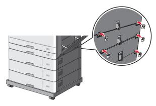
**b** Secure the brackets with screws.
