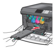
7 Using both hands, push the sides of the internal cover firmly until it *clicks* into place.
