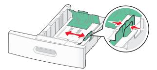
**3** Unlock the length guide, squeeze the length guide tab inward as shown, and slide the guide to the correct position for the paper size being loaded.
