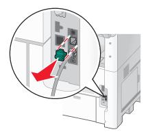
**4** Connect the other telephone cord to a telephone, and then plug it into the EXT port into the printer.
