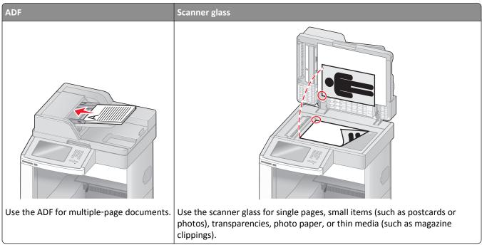
The scanner lets you scan documents directly to a computer or to a flash drive. The computer does not have to be directly connected to the printer for you to receive Scan to PC images. You can scan the document back to the computer over the network by creating a scan profile on the computer, and then downloading the profile to the printer.
