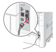
**3** Connect the other end of the telephone cord into the N slot of an active telephone wall jack.
