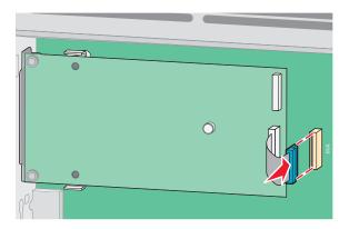
**12** If a printer hard disk was previously installed, then attach the printer hard disk to the ISP. For more information, see "Installing a printer hard disk" on page 32.
