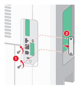
**4** Insert the fax card and attach the two provided screws to secure the fax card mounting bracket.
