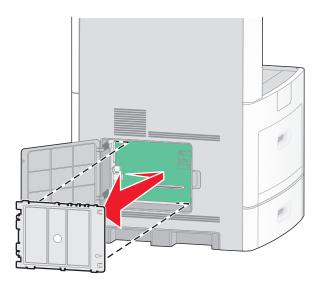
**4** Use the illustration below to locate the appropriate connector.
