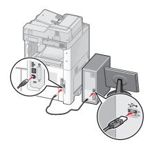
**Note:** After the printer is configured, the software will instruct you to disconnect the temporary USB cable so you can print wirelessly.
