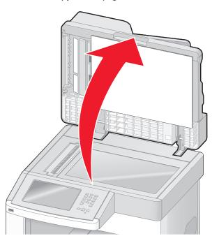
**5** Open the bottom ADF door, and then remove any jammed pages.
