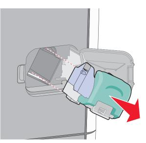
**4** Use the metal tab to lift the staple guard, and then remove any loose staples.
