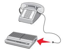
**5** Connect a third telephone cord from the answering machine to the EXT port in of the printer.
