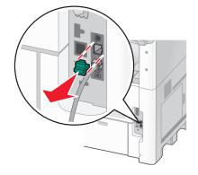
**2** Connect your telecommunications equipment directly to the EXT port in on the back of the printer.
