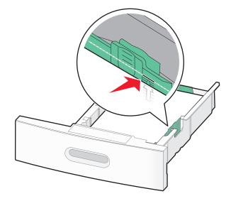
**6** If necessary, adjust the paper guides to lightly touch the sides of the stack, and lock the length guide for the paper sizes indicated on the tray.
