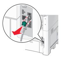
**Note:** Once this plug is removed, any country- or region-specific equipment you connect to the printer by way of the adapter, as shown, will not function properly.
