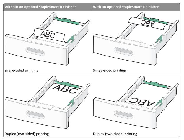
**Note:** Notice the maximum fill line on the side of the tray which indicates the maximum height for loading paper. Do not overload the tray.
