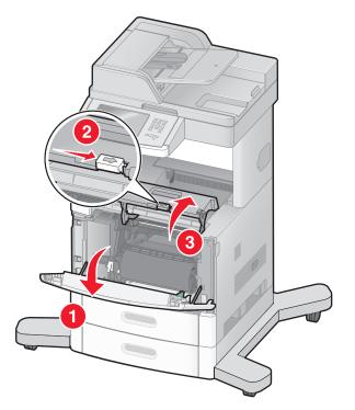
**4** Lift and pull the print cartridge out of the printer.
