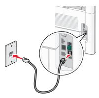
**3** Remove the protective plug from the EXT port m of the printer.
