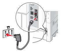
**4** If you would like to use the same line for both fax and telephone communication, connect a second telephone line (not provided) between the telephone and the F slot of an active telephone wall jack.
