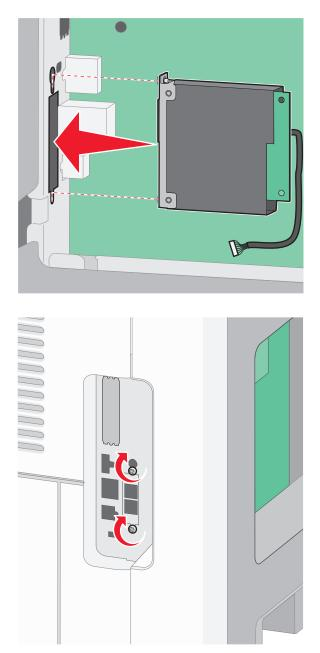
**5** Insert the plug of the fax card interface cable into the receptacle of the system board.
