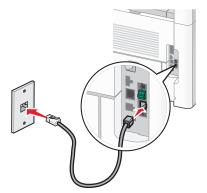
**3** Remove the protective plug from the EXT port  $\widehat{\blacksquare}$  of the printer.
