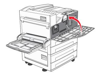
**Note:** After you insert the photoconductor and close all the doors, the printer performs a motor cycle and clears the Replace Photoconductor warnings.
