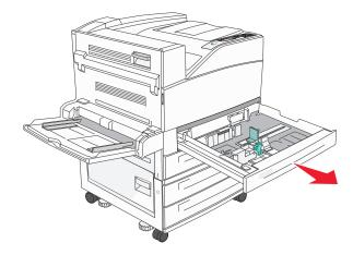
2 Squeeze and slide the width and length guides to the correct positions for the paper size being loaded.
