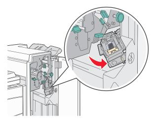
**3** Firmly pull the colored tab to remove the staple cartridge.
