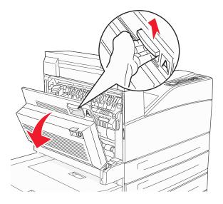
**2** Open Door E by pushing the release latch and lowering the door.
