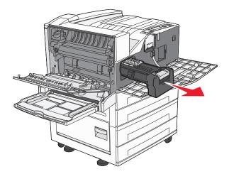
Place the photoconductor on a flat, clean surface.
