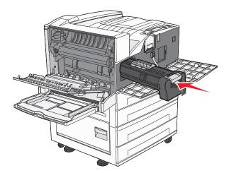
The photoconductor clicks into place when correctly installed.
