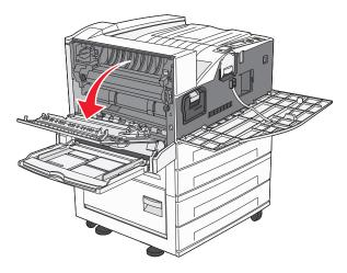
4 Pull the photoconductor out of the printer.
