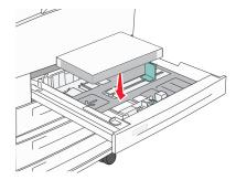
By default, the printer is set to recognize letter- or A4-size paper loaded in the long-edge orientation. If you want to load letter- or A4-size paper in the short-edge orientation, make sure you enable "Short Edge printing".
