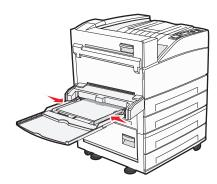
7 From the printer control panel, set the Paper Size and Paper Type for the multipurpose feeder (MP Feeder Size and MP Feeder Type) based on the paper you loaded.
