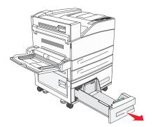
2 Squeeze the length guide tab inward as shown, and slide the guide to the correct position for the paper size being loaded.
