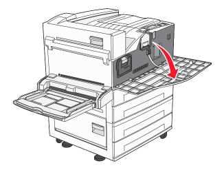
**3** Grasp the handle and pull out the cartridge.
