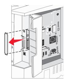
4 Align the connector on the internal print server or port interface card with the connector on the system board.
