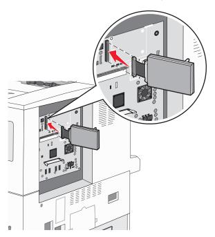
**6** Flip the hard disk over, and then press the three posts on the mounting plate into the holes on the system board. The hard disk *snaps* into place.
