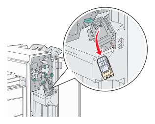
**4** Use the metal tab to lift the staple guard, and then pull out the sheet of staples. Discard the entire sheet.
