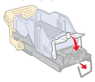
**7** Push the cartridge holder firmly into the stapler until the holder clicks into place.
