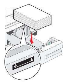
**Note:** Make sure the paper is below the maximum fill line on the rear guide. Overloading may cause jams.
