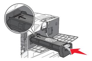
**7** Remove the tape from the top of the photoconductor.
