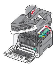
4 Remove the toner cartridge by lifting the handle, and then gently pulling away from the imaging kit.
