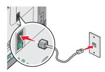
**3** Remove the protective plug from the bottom EXT port  $\widehat{\ }$  of the printer.
