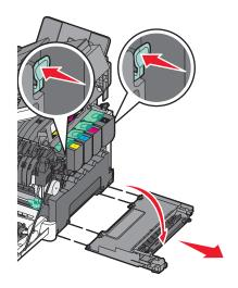
**5** Press the green levers on each side of the waste toner bottle, and remove it.
