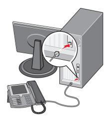
**5** Connect a third telephone cord from the computer modem to the bottom EXT port  $\widehat{\underline{\ }}$  of the printer.
