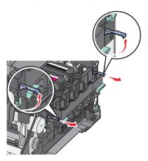
**7** Press down on the blue levers, grasp the green handles on the sides, and then pull the imaging kit out.
