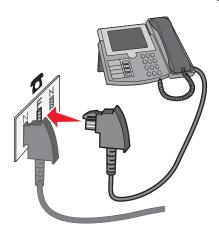
4 If you would like to use the same line for recording messages on your answering machine, then connect a second telephone line (not provided) between the answering machine and the other N slot of the active analog telephone wall jack.
