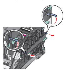
7 Press down on the blue levers, grasp the handles on the sides, and then pull the imaging kit out.
