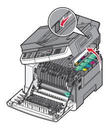
**3** Remove the toner cartridges by lifting the handles, and then gently pulling away from the imaging kit.
