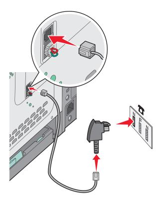
**3** If you would like to use the same line for both fax and telephone communication, then connect a second telephone line (not provided) between the telephone and the F slot of an active analog telephone wall jack.
