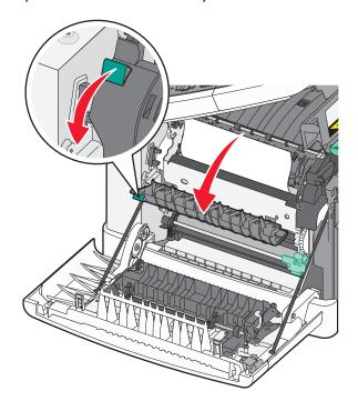
**3** Hold the fuser cover down, and then remove the jammed paper. The fuser cover closes when released.
