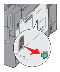
**2** Connect your telecommunications equipment directly to the bottom EXT port  $\widehat{}$  on the back of the printer.
