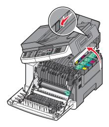
**3** Remove the toner cartridges by lifting the handles and then gently pulling away from the imaging kit.
