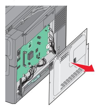
**4** Locate the appropriate connector on the system board.
