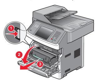
**4** Lift the flap at the front of the printer, and then remove any jammed sheets.
