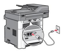
**3** Remove the protective plug from the printer EXT port :
