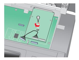
**9** Attach the two provided screws to secure the ISP mounting bracket to the system board cage.
