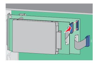
To install a printer hard disk directly onto the system board:
