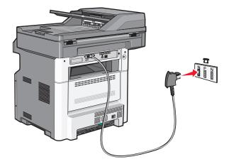
**4** If you would like to use the same line for both fax and telephone communication, then connect a second telephone line (not provided) between the telephone and the F slot of an active analog telephone wall jack.
