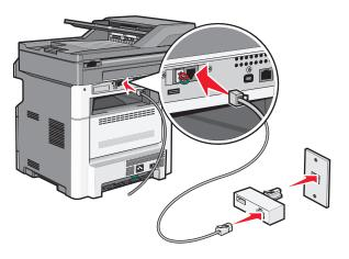
**3** Connect the answering machine or telephone to the adapter. Use one of the following methods:
