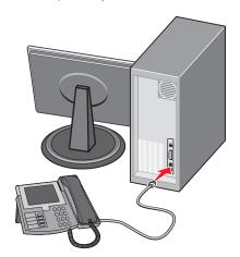
**5** Connect an additional telephone cord (not provided) from the computer modem to the printer EXT port  $\stackrel{\frown}{=}$ .
