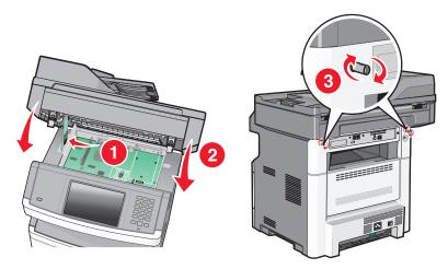
**Warning—Potential Damage:** Make sure the system board is locked to prevent possible damage to the printer if it is moved.
