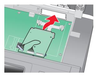
7 Lower the ISP toward the plastic tee until the ISP is seated between the guides of the plastic tee.
