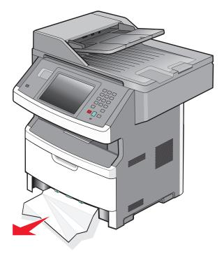
**3** If you do not see the jam, open the front door, and then remove the photoconductor kit and toner cartridge.
