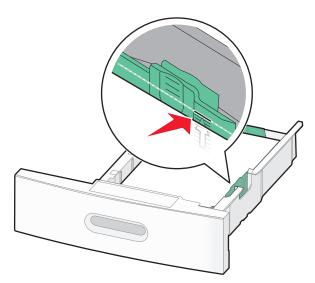
**6** If necessary, adjust the paper guides to lightly touch the sides of the stack, and lock the length guide for the paper sizes indicated on the tray.
