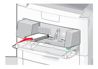
Note: Do not exceed the maximum stack height by forcing paper under the stack height limiter.
