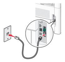
**3** Remove the protective plug from the EXT port of the printer.
