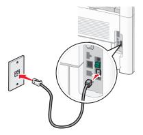
**3** Remove the protective plug from the EXT port for the printer.
