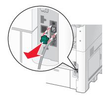
**4** Connect the other telephone cord to a telephone, and then plug it into the EXT port of the printer.
