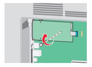
**9** Attach the two provided screws to secure the ISP mounting bracket to the system board cage.
