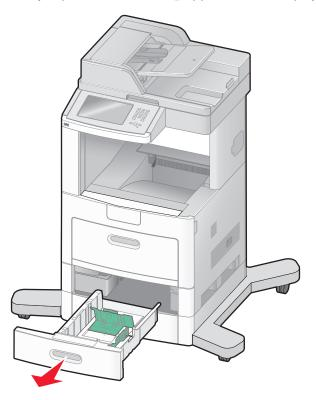
**2** Squeeze the width guide tab inward as shown, and move the width guide to the correct position for the paper size being loaded.
