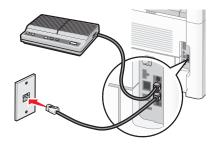
**Note:** Once this plug is removed, any country- or region-specific equipment that you connect to the printer by way of the adapter, as shown, will not function properly.
