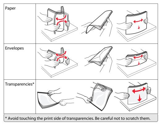
**5** Load the paper or specialty media. Slide the stack gently into the multipurpose feeder until it comes to a stop.
