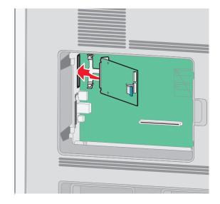
7 Lower the ISP toward the plastic tee until the ISP is seated between the guides of the plastic tee.
