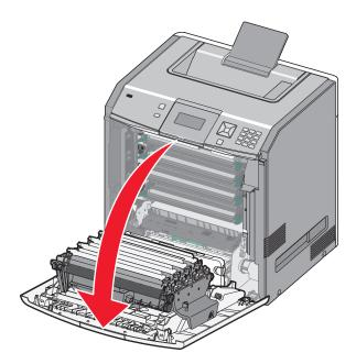
**Warning—Potential Damage:** To avoid overexposing the photoconductor units, do not leave the front door open for more than 10 minutes.
