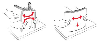
• Hold transparencies by the edges, and then fan them. Straighten the edges on a level surface.
