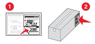
**8** Insert the new waste toner box into the printer.
