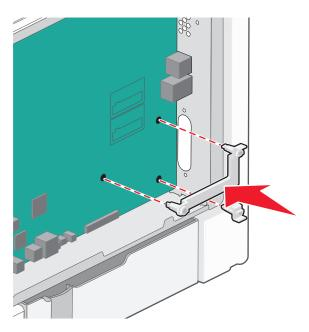
**6** Install the ISP on the plastic tee. Angle the ISP over the plastic tee, and approach the plastic tee so that any overhanging connectors will pass through the ISP opening in the system board cage.
