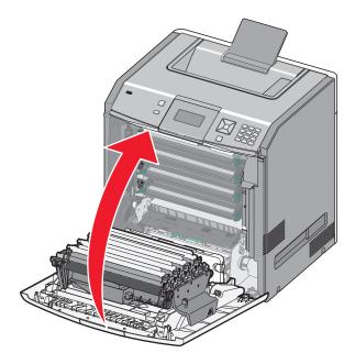
**Note:** Make sure each cartridge is fully pushed in. If a cartridge is not installed correctly, the printer may issue a <color> Cartridge Missing message, where <color> is Black, Cyan, Magenta, or Yellow. The printer may also issue the message Close front door.
