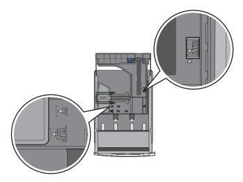
2 Squeeze the width guide tabs as shown, and then slide the guide to the correct position for the size of paper being loaded.
